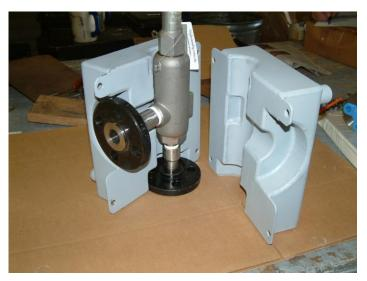
Flow Fab Clamp-On Jackets are a form fitting fabrication for piping components, such as valves, pumps, fittings, meters and other items. Steam or hot oil may be used as a heating medium. They offer maximum efficiency for application of heat to those items.
