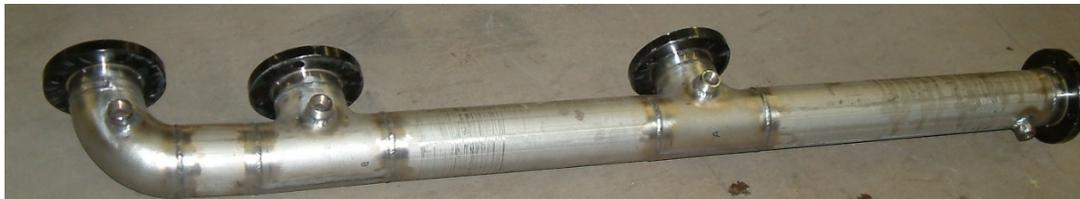
Jacketed pipe consists of a core pipe for conveying viscous fluids, with an outer jacket pipe. The annular chamber between the two pipes is used to heat the inner pipe with steam or hot oil.
